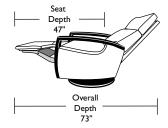
Note: All height dimensions represent recliner at lowest position of swivel base or with fixed leg option. The height of recliners with swivel base option can increase approximately 2-1/4" by simply rotating the recliner counter-clockwise.
